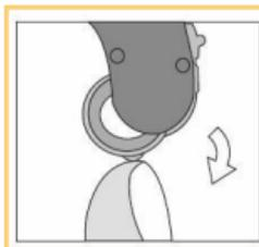
Push the nail grip downwards to swing open the battery compartment. The nail grip is located below the power switch at the bottom of the hearing aid.
